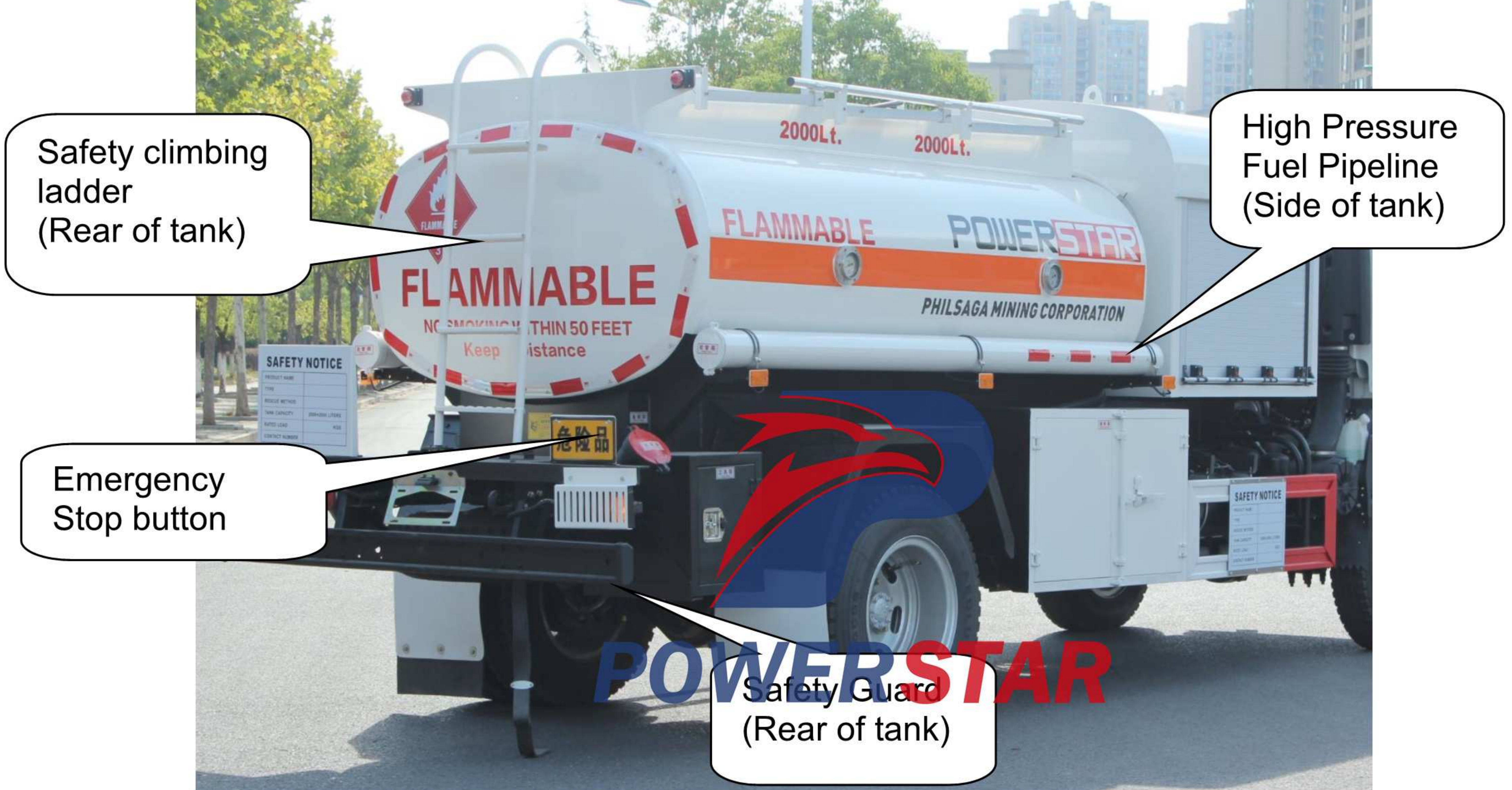
Rear of the Tank: Rear Climbing Ladder, Submarine Emergency Stop Button & Pipeline Container
